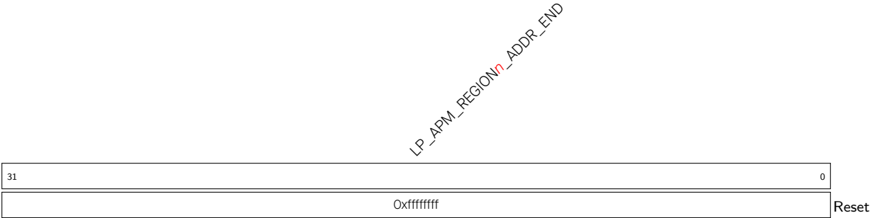
Register 13.31. LP_APM_REGION n _ADDR_END_REG ( n : 0-7) (0x0008+0xC* n )
