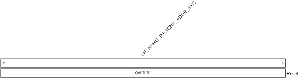
Register 13.47. LP_APMO_REGION n _ADDR_END_REG ( n : 0-7) (0x0008+0xC* n )
