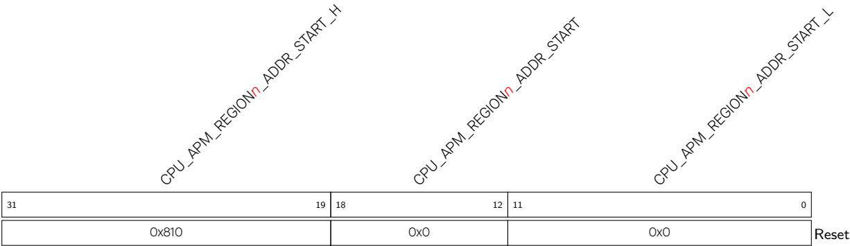
Register 13.58. CPU_APM_REGION n _ADDR_START_REG ( n : 0-7) (0x0004+0xC* n )
