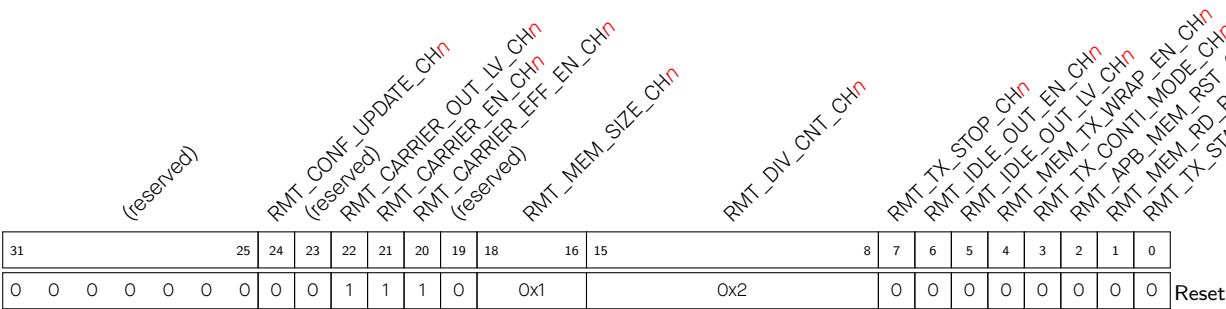
Register 32.2. RMT_CHnCONFO_REG (n: 0-1) (0x0010+0x4*n)
