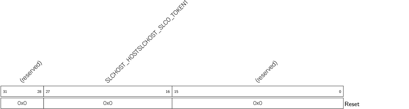
Register 29.50. SLCHOST_SLC0HOST_TOKEN_RDATA_REG (0x0044)
