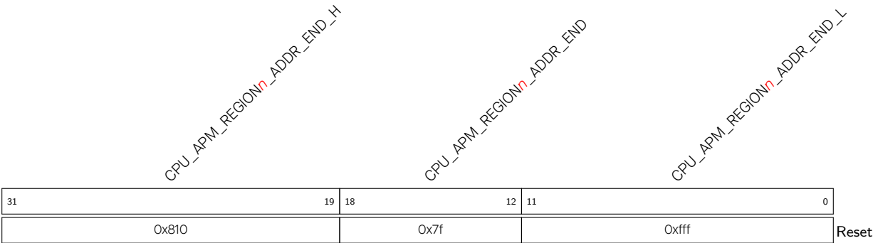
Register 13.59. CPU_APM_REGION n _ADDR_END_REG ( n : 0-7) (0x0008+0xC* n )
