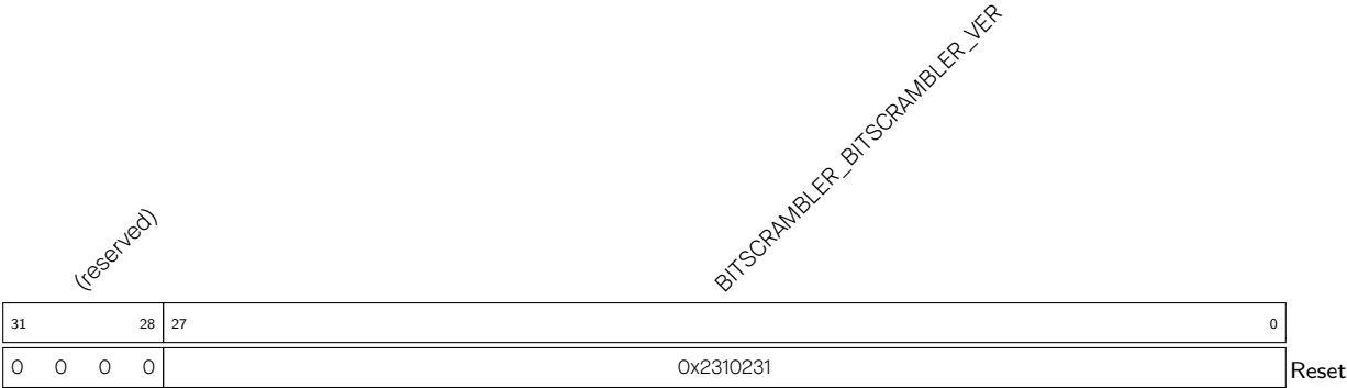
Register 34.16. BITSCRAMBLER_VERSION_REG (0x00FC)
