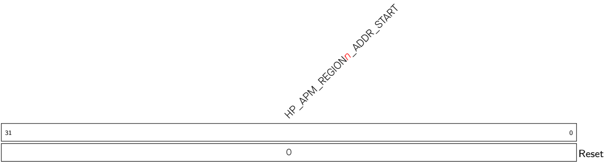
Register 13.2. HP_APM_REGION n _ADDR_START_REG ( n : 0-15) (0x0004+0xC* n )
