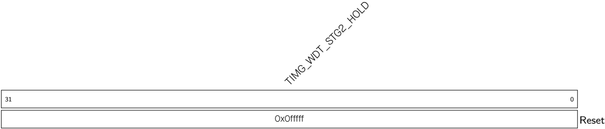
Register 10.14. TIMG_WDTCONFIG4_REG (0x0058)
