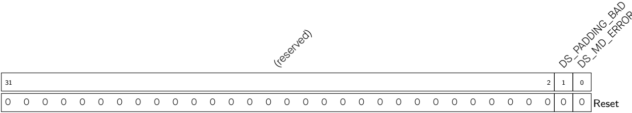
Register 21.6. DS_QUERY_CHECK_REG (0x0E14)
