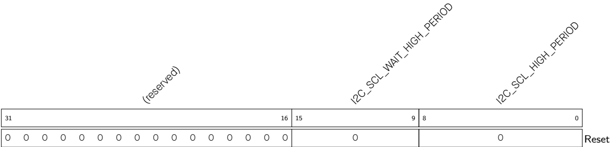
Register 26.4. I2C_SCL_HIGH_PERIOD_REG (0x0038)
