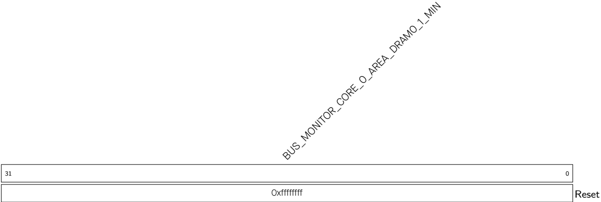
Register 14.19. BUS_MONITOR_CORE_O_AREA_DRAMO_1_MIN_REG (0x0018)
