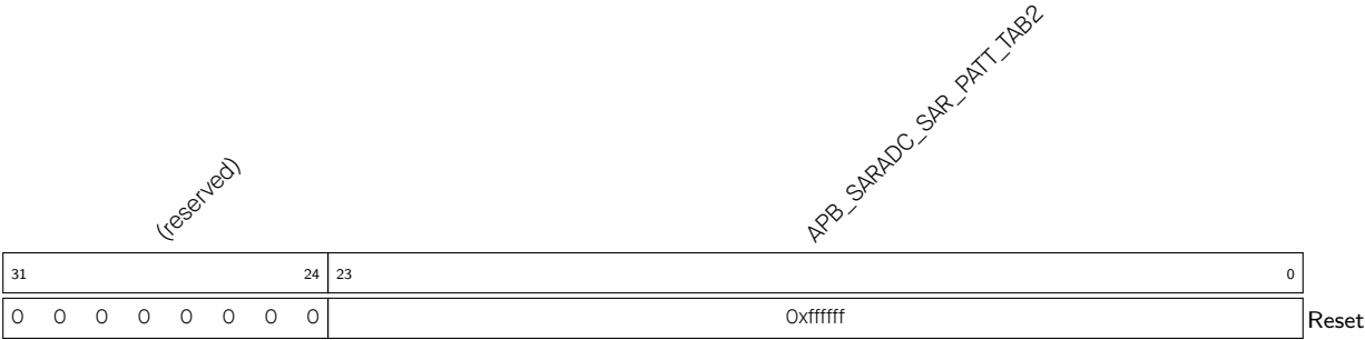
Register 36.5. APB_SARADC_SAR_PATT_TAB2_REG (0x001C)
