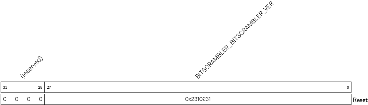
Register 34.16. BITSCRAMBLER_VERSION_REG (0x00FC)
